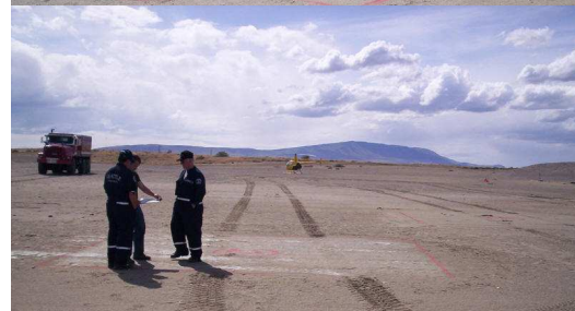
In addition to particle lockdown, IsoFIX also withstands extreme vehicle traffic. A 23-ton fire truck does not break the elastomeric crust of the IsoFIX- treated pad (above).
